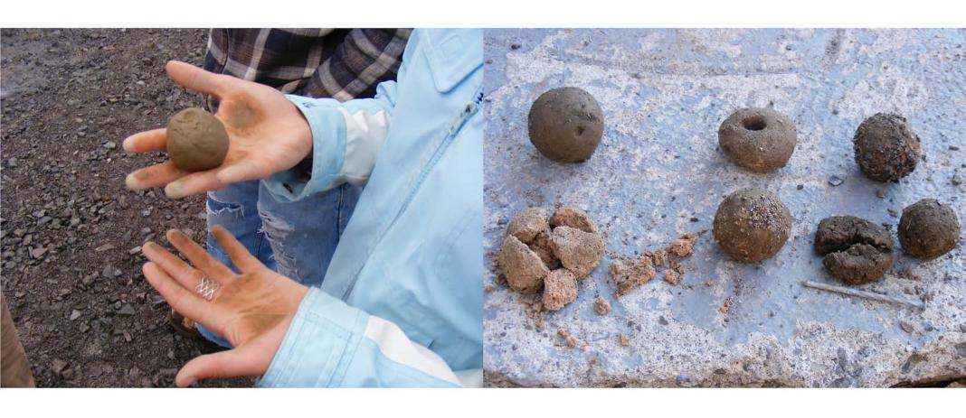
Many different fill materials can work inside an earthbag. Fill shouldn't be rich in binder (whether clay, lime or cement), but mostly aggregate with just enough binder to compact well.
