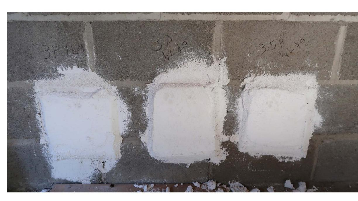
**Insulating plaster test patches**
