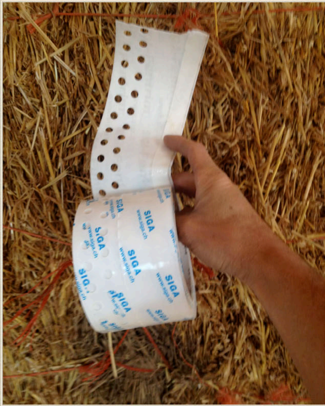
Our first experience using Siga tape to air seal at junctions was a success that we will repeat on future buildings.
