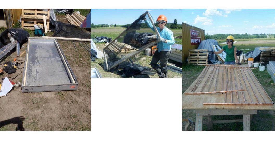
Home made solar hot water and hot air collectors are built from used panels. Kara prepares the double screen innards of the air units and Melissa solders up pipes for the water units.
