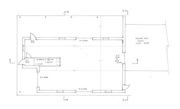
The section drawing shows the quonset hut root cellar sharing the same grade with the processing facility. The main floor plan shows the open washing/processing area.
